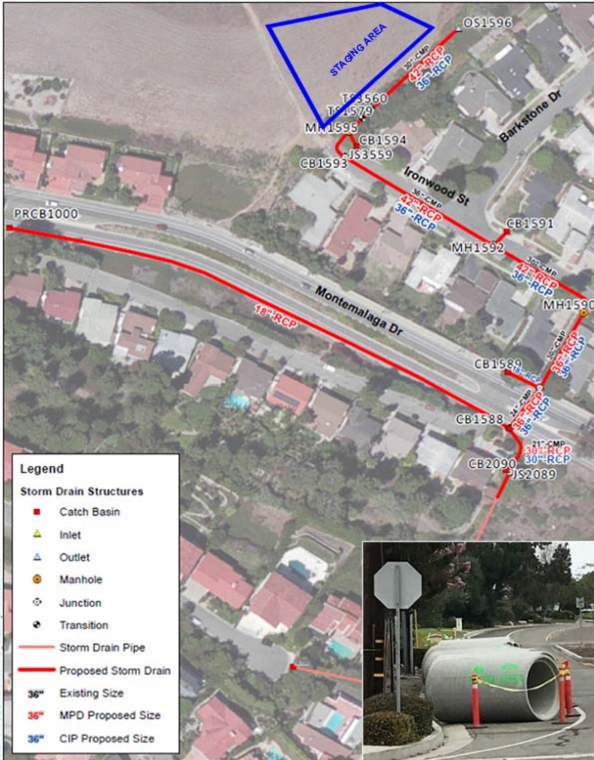
Figure 1. Proposed Work Location and Pipe Sizes
