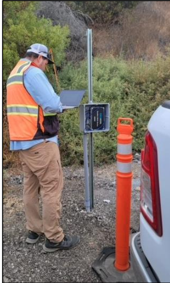
Inclinometer data logging at the (E-1-9) borehole site (left) and drilling operations at the E-2 borehole locations (right)
