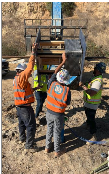
Recovery of Shapearray Inclinometer from Borehole A-4N (Left) and Winterization Work in Altamira Canyon (Right)
