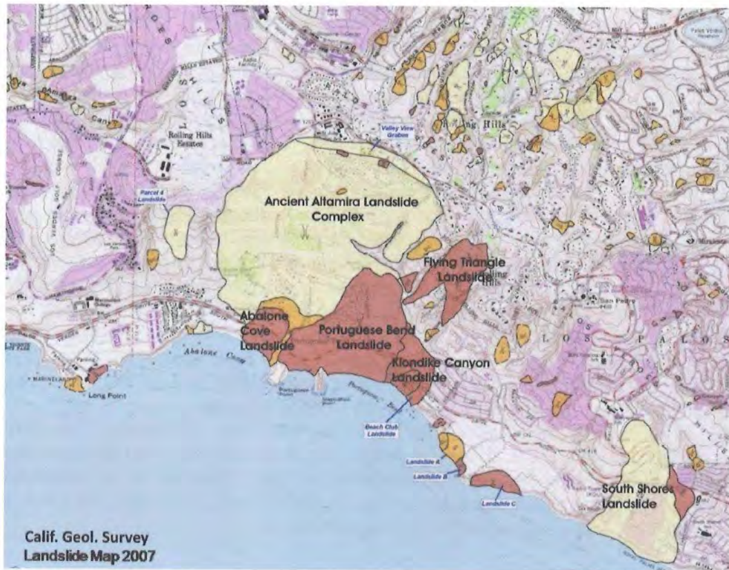
Figure 1. Landslide map of a portion of the south flank of the Palos Verdes Peninsula prepared by the California Geological Survey (2007). The major and some minor landslides are identified. Light yellow indicates that the landslide is inactive, red is active and orange is dormant.
